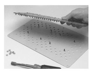
The LED circuit board is held to the mask by several nuts, which you can remove using a 3/8-inch nut driver. On outdoor displays the thick conformal coating can be messy, as the lock washers on the nuts dig into the coating and knock pieces of it away. Be careful to keep the whole assembly right side up when you return it to the display cabinet.
