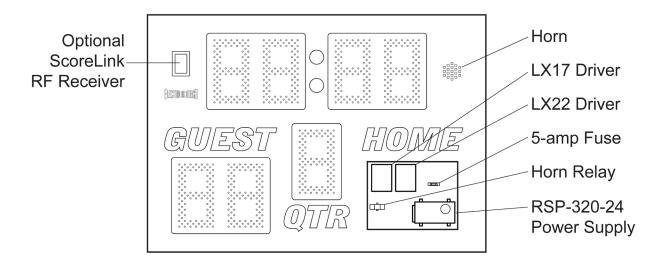
If your scoreboard system includes a ScoreLink wireless data kit, the receiver unit will be located in the upper left corner of the display face. The internal Horn will be mounted in the upper right corner. To access the Horn for service, remove the Period Clock Seconds digit assembly.
